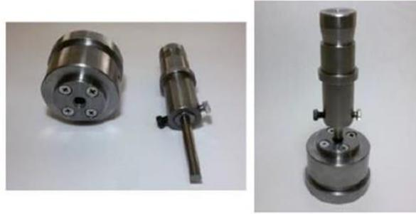
**Figure 2.** Mold and punch used in pressing
