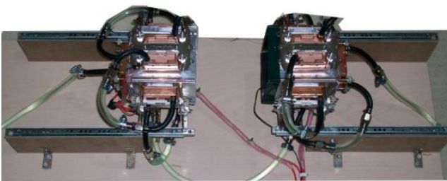
Figure 3. Thermoelectric cooling container
