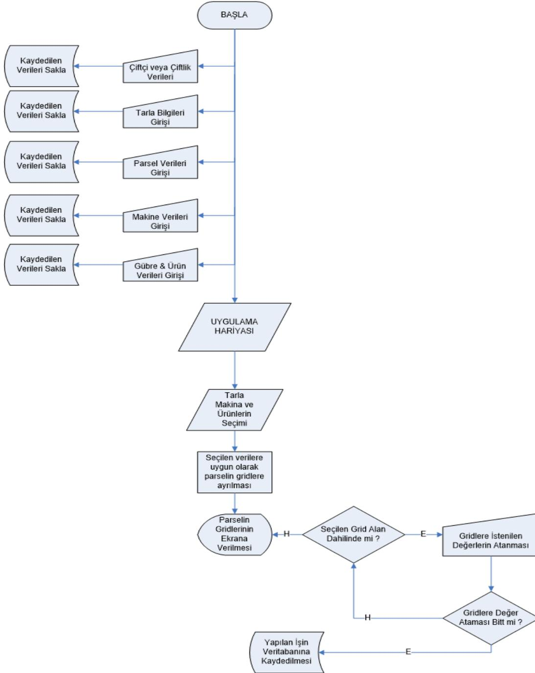
**Figure 10.** Algorithm of the variable rate fertilisation software
