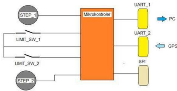
**Figure 4.** Block diagramme of the new designed variable rate controller
