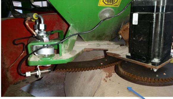
**Figure 3.** Connection of the limit switch to the system
