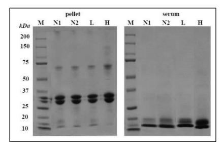
**Fig. 1.** SDS-PAGE profiles of yogurt samples (Lane M represents the standard marker). Pellets comprised CN fractions and serums comprised WP fractions: N1: national yogurt1, N2: national yogurt2, L: local yogurt, H: homemade yogurt
