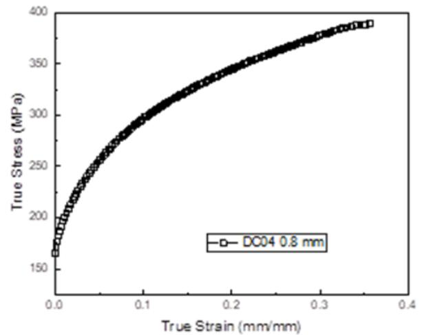
Figure 3. Flow curve of 0.8 mm DC04 EN10130
