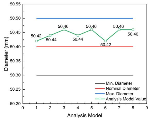
**Figure 11.** Outer diameter results according to analysis models
