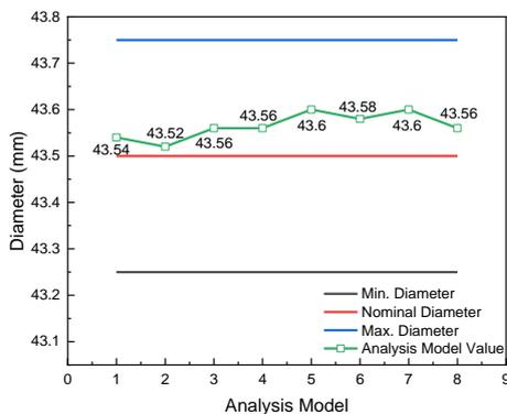
**Figure 9.** Hole diameter results according to analysis models
