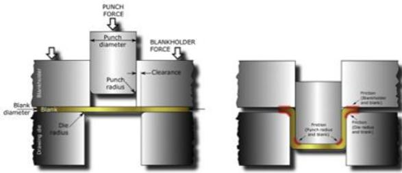
Figure 1. Schematic sheet metal forming setup [12]
