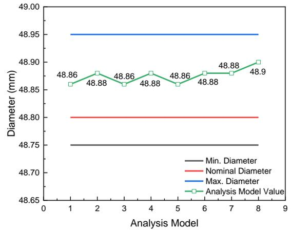
**Figure 10.** Inner diameter results according to analysis models
