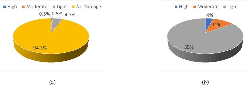
**Figure 10.** Damage Distribution of Investigated Buildings: a) Total Damaged Buildings, b) RC Damaged Buildings
