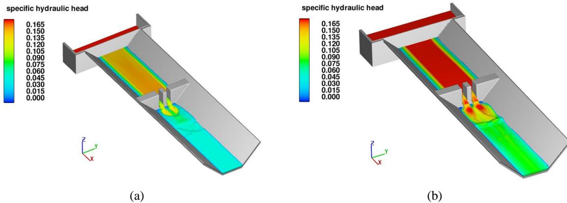
**Figure 12.** 3D distribution of specific hydraulic head for E-weir (a)  $Q=30 \text{ m}^3/\text{h}$  (b)  $Q=66 \text{ m}^3/\text{h}$
