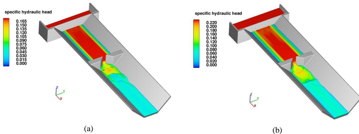
**Figure 13.** 3D distribution of specific hydraulic head for V-weir (a)  $Q=30 \text{ m}^3/\text{h}$  (b)  $Q=66 \text{ m}^3/\text{h}$
