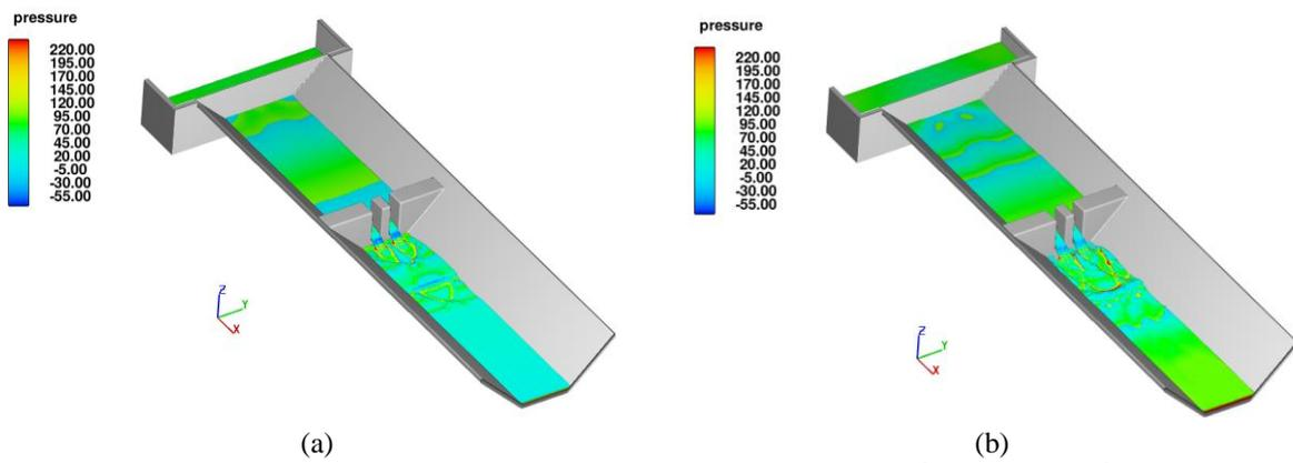
Figure 9. 3D distribution of pressure for E-weir (a)  $Q=30 \text{ m}^3/\text{h}$  (b)  $Q=66 \text{ m}^3/\text{h}$
