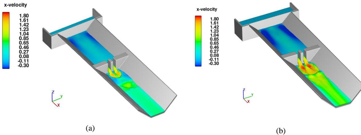
**Figure 6.** 3D distribution of x velocity for E-weir (a)  $Q=30 \text{ m}^3/\text{h}$  (b)  $Q=66 \text{ m}^3/\text{h}$
