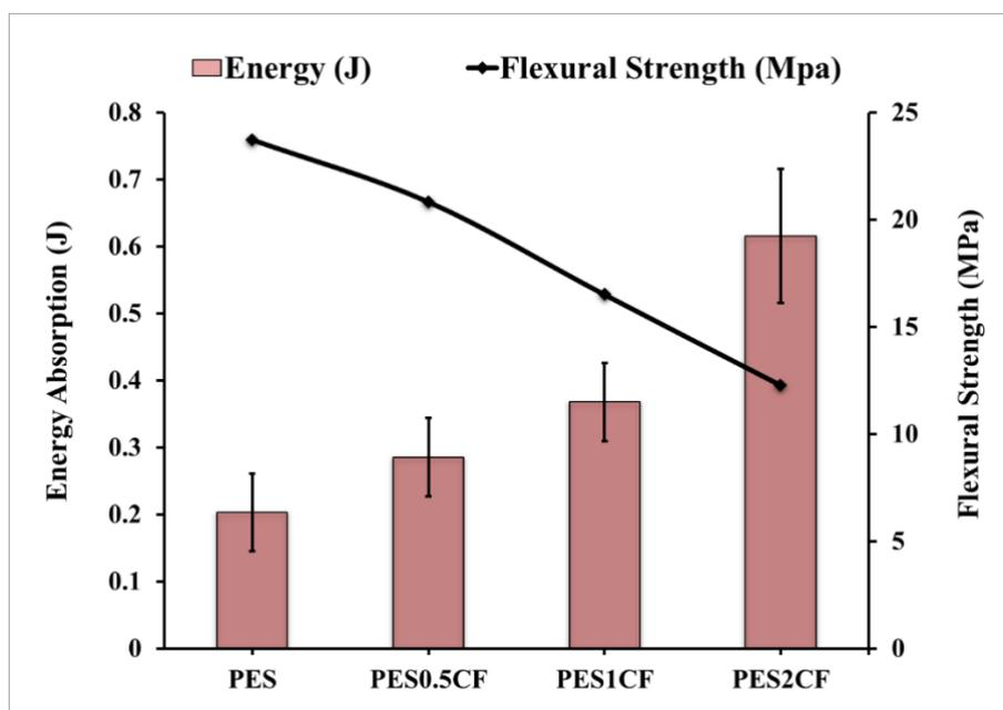
*Figure 3. Flexural Strength and energy absorption of samples.*
