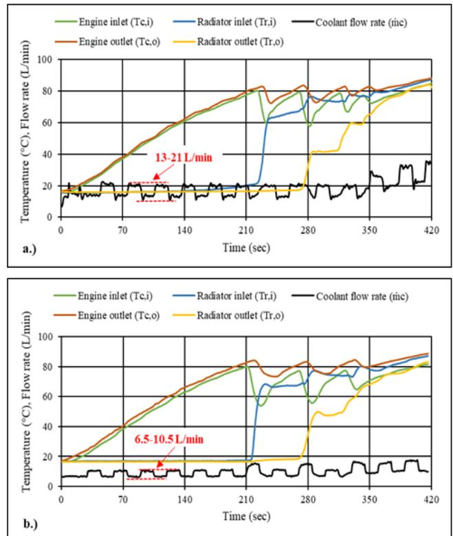
Figure 3 Instantaneous variations of coolant temperature and coolant flow rate at 2000-3000 rpm / 25% load, [a.) MPICS - b.) EPICS].
