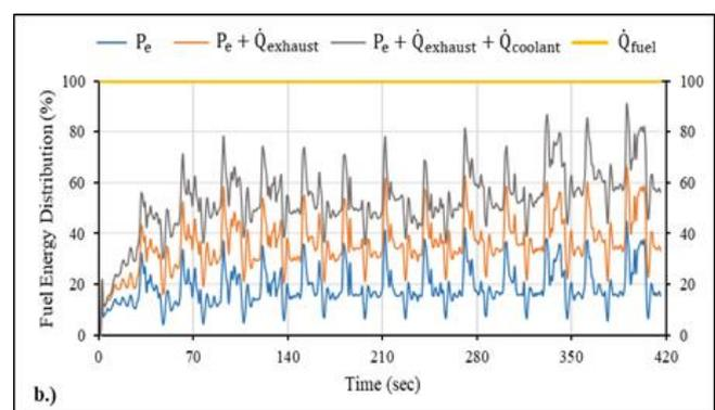
Figure 6 Instantaneous energy distributions of fuel energy at 2000-3000 rpm / 25% load, [a.) MPICS - b.) EPICS].
