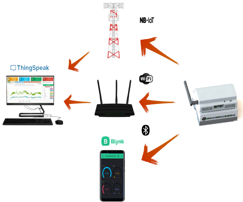
Figure 4. The connectivity options of designed smart meter for remote server access
