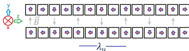
**Figure 1.** Ideal planar undulator in the Halbach configuration.
