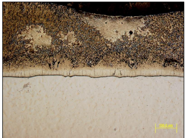
Figure 4. Micrograph of a Partially Matt, Partially Glossy Galvanized (GGA, 2021)
