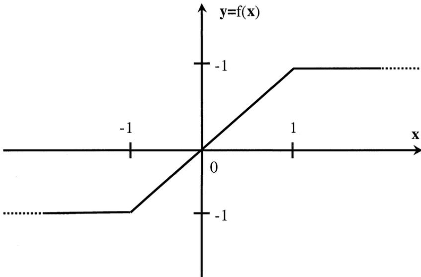
Figure 4. Piece-wise Linear Output Characteristics of CNN cell.
