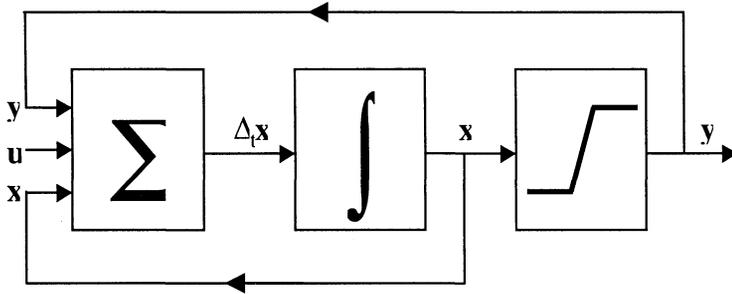
Figure 3. CNN model input-output relationship.
