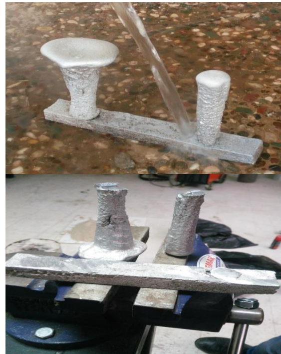
Figure 3. Separating the excesses and sprues of produced cast samples
