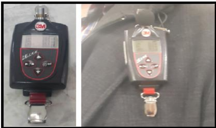
Figure 4. Personal noise exposure measuring device
