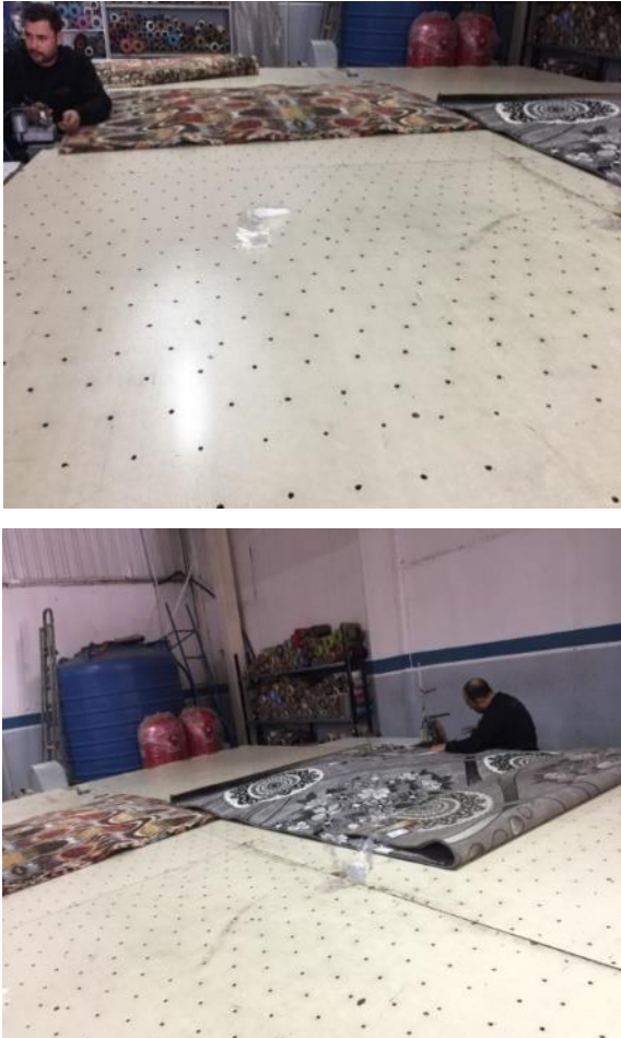
Figure 11. Pneumatic table and pneumatic table working area
