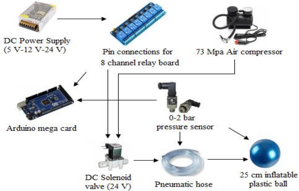
Figure 4. Block scheme of the experimental setup.
