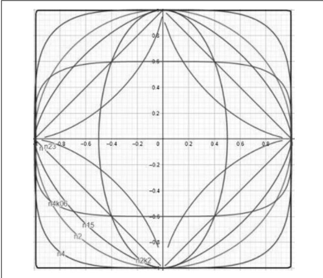
**Figure 1.** Super ellipses for different parameters. **n100** (approximately square):  $n=100$ ,  $a=b=1$ ; **n4** (squircle):  $n=4$ ,  $a=b=1$ ; **n2** (circle):  $n=2$ ,  $a=b=1$ ; **n15** (curved rhombus):  $n=1.5$ ,  $a=b=1$ ; **n1** (rhombus):  $n=1$ ,  $a=b=1$ ; **n23** (asteroid):  $n=2/3$ ,  $a=b=1$ ; **n4k06** (super ellipse):  $n=4$ ,  $a=1$ ,  $b=0.6$ ; **n2k2** (ellipse):  $n=2$ ,  $a=0.5$ ,  $b=1$ .
