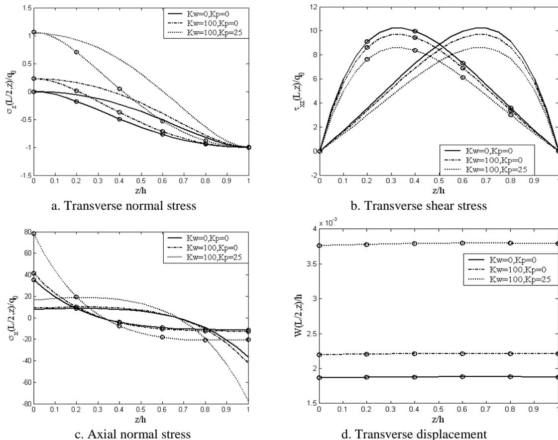
Fig.3. Variation of stresses and displacement across the thickness, CS,  $L/h=10$
