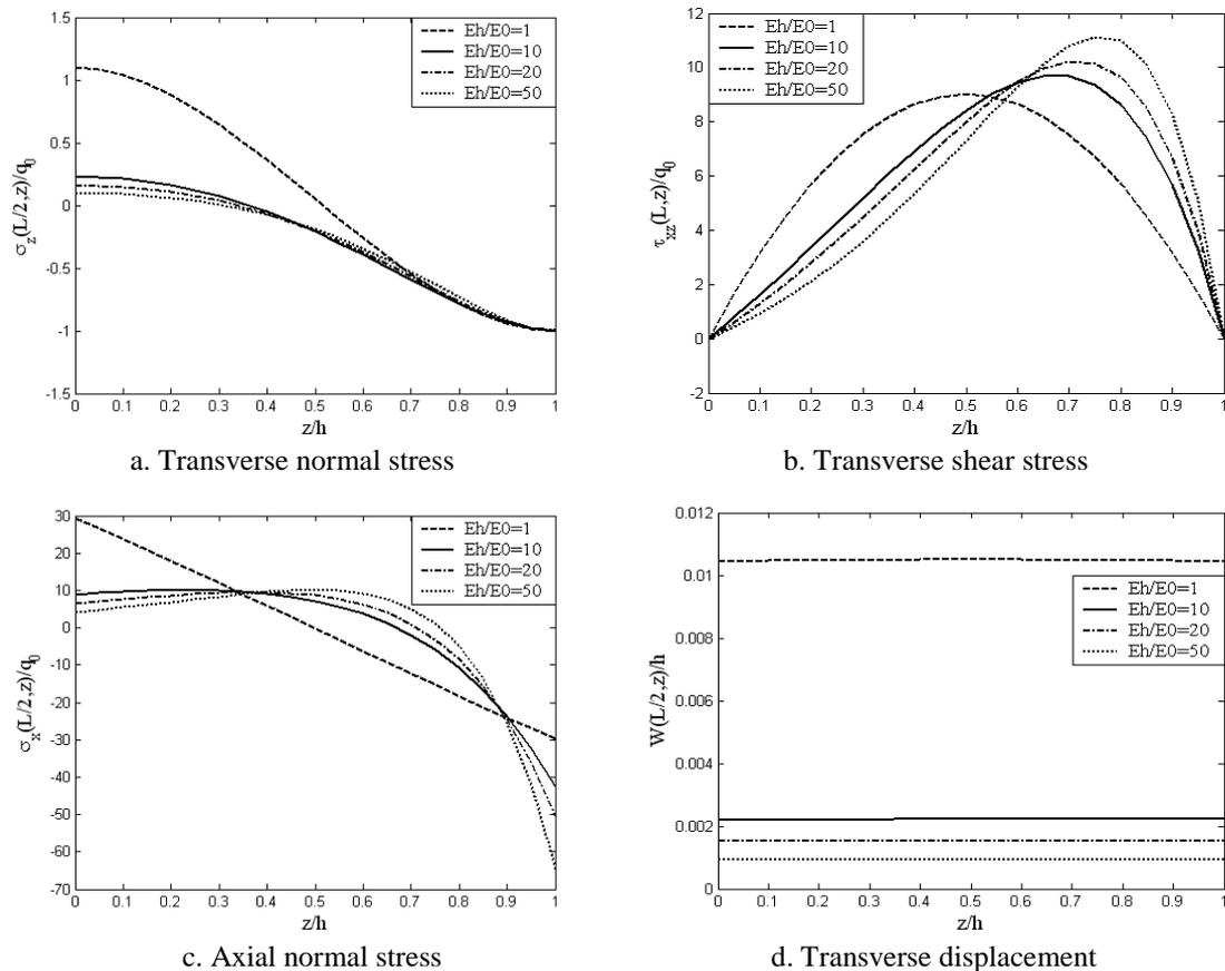
Fig.5. Effect of gradient index on mechanical parameters for FGM beam, CS,  $L/h=10, K_w=100, K_p=25$
