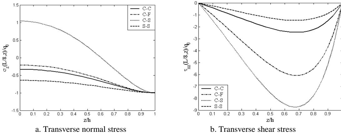
Influence of edges conditions in axial stress near the outer surface is much more than the lower position in thickness direction, but for transverse normal stress near the lower surface, it is much more than the outer surface. Distribution of transverse displacement across the thickness in contrast with the other quantities is constant.
