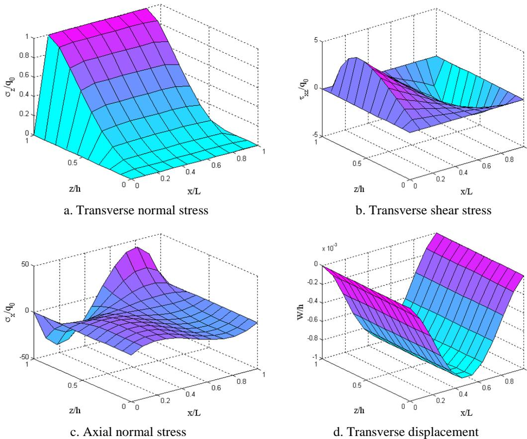
Fig.7. Mechanical parameters in two directions for FGM beam, CC,  $K_w = 0$ ,  $K_p = 0$
