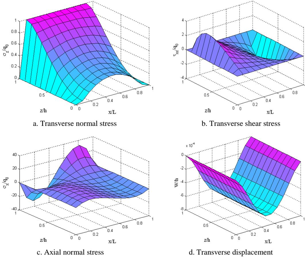
Fig.8. Mechanical parameters in two directions for FGM beam, CC,  $K_w = 100$ ,  $K_p = 25$
