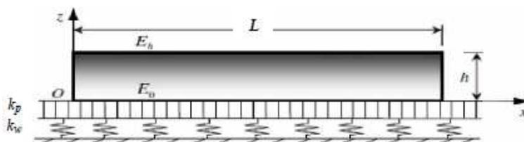
Fig.1 .Functionally graded beam on tow parameter elastic foundation
