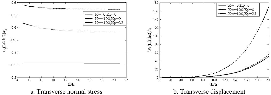
Fig.4. Effect of aspect ratio on transverse normal stress and displacement for FGM beam, CF
