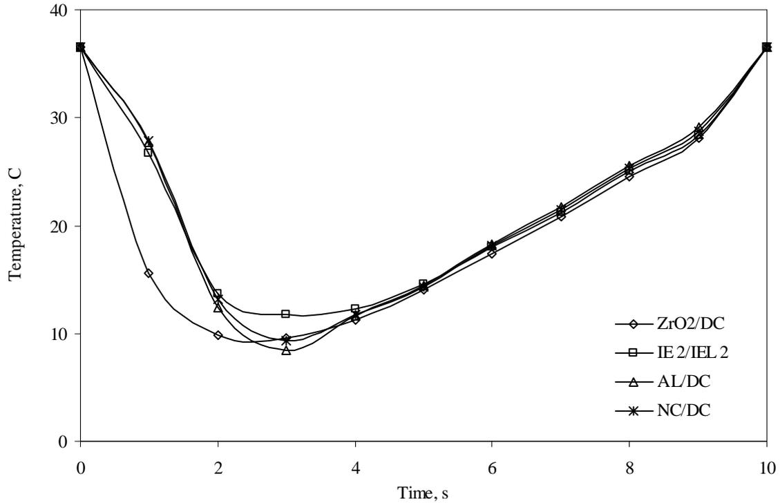
Fig. 5. Temperature changes depending on time at Node B caused by cold liquid
