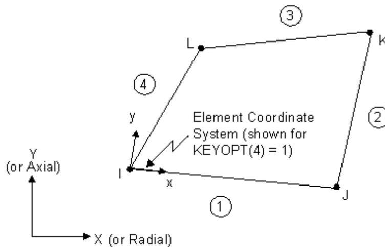
Fig. 2. Coupled-field solid element type (PLANE13)
