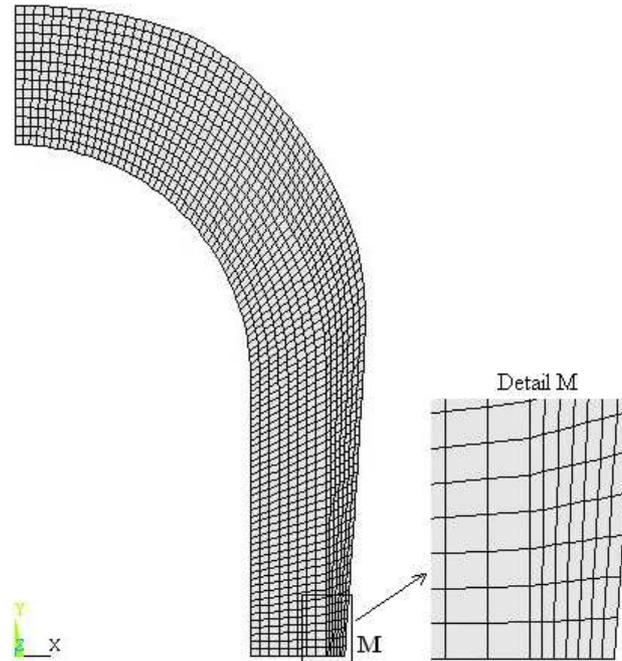
Fig. 3. The axisymmetric finite element model of the crown structure
