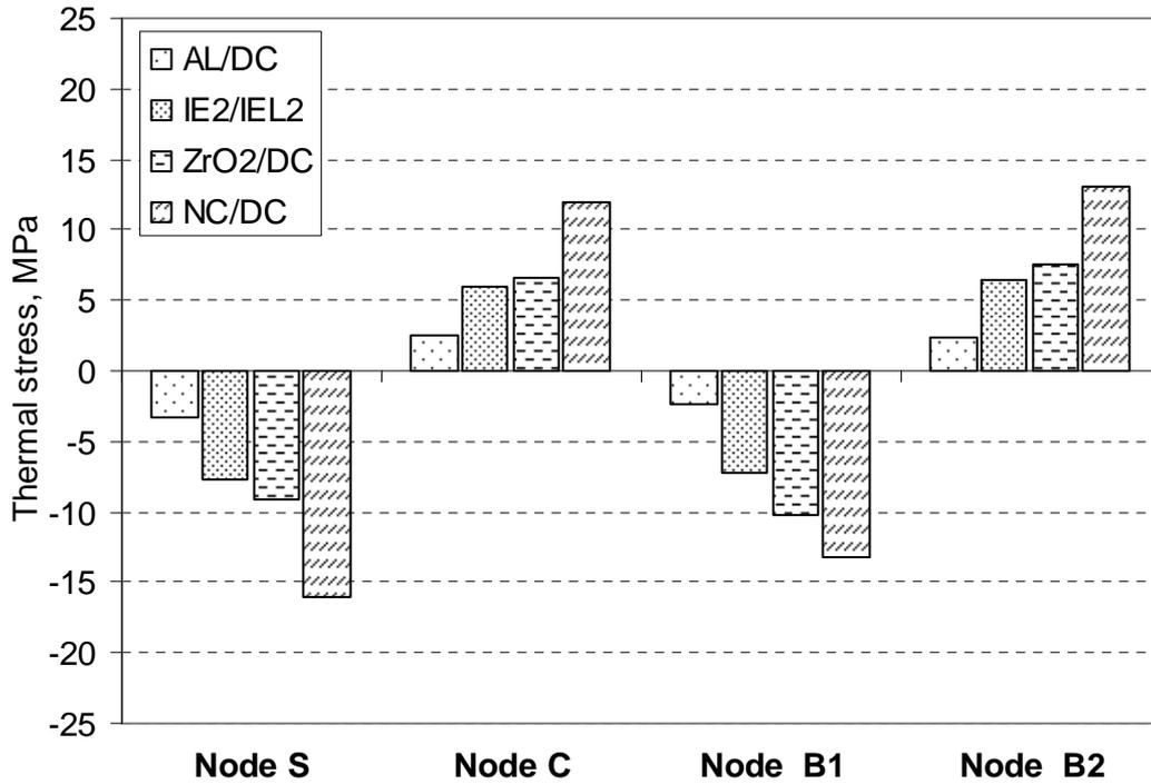
Fig. 8. The maximum values of thermal stresses at selected nodes caused hot liquid
