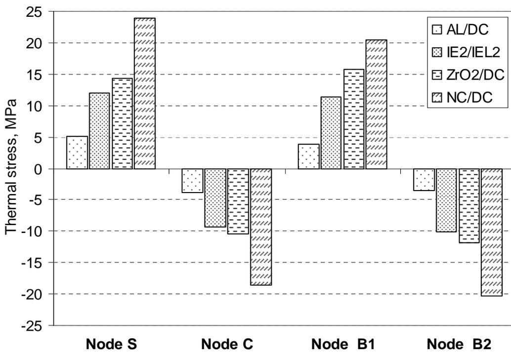
Fig. 9. The maximum values of thermal stresses at selected nodes caused cold liquid
