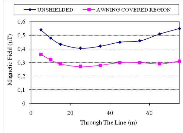
Fig.6. Magnetic field measurements through the line at North Part of Varsak Shopping Centre
