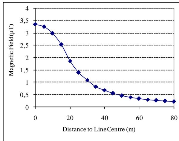
Fig.3. Magnetic field measurement with respect to distance from 380kV power lines.
