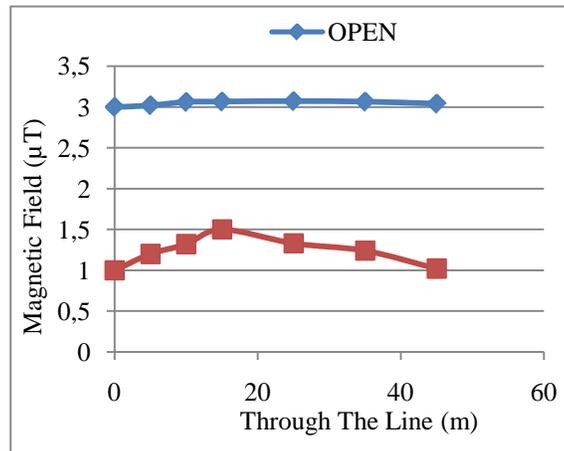
Fig.7. Magnetic field measurements through the line at South Part of Varsak Shopping Centre
