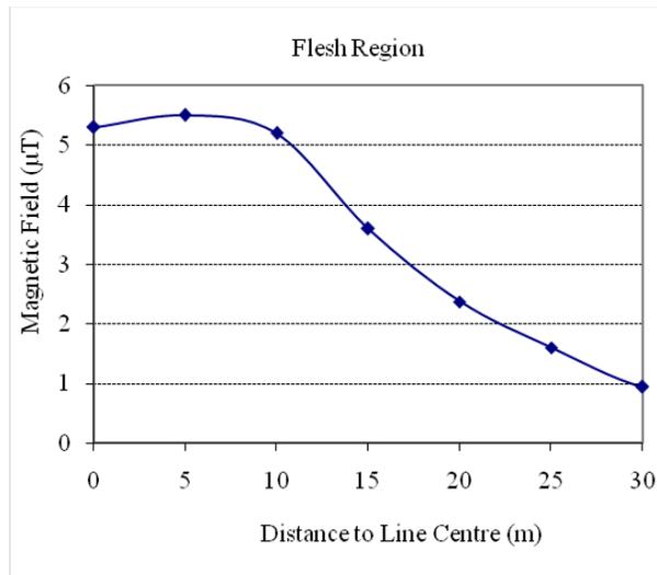
Fig.5. Magnetic field measurements with respect to distance from power lines at flesh region
