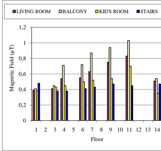
Fig.8. Magnetic field measurements at 15 floors apartment.
