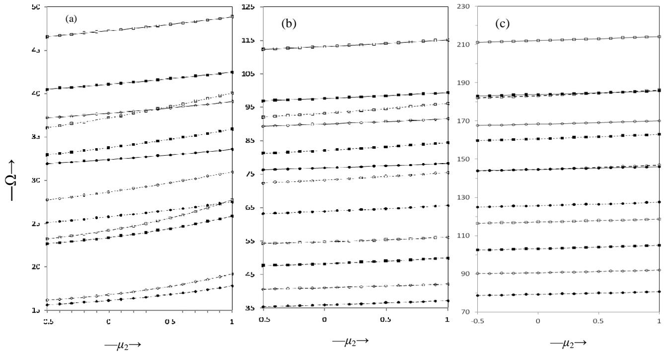
Fig. 4: Frequency parameter for C-C, C-S and C-F plates vibrating in (a) first mode (b) second mode and (c) third mode, for  $a/b = 1$ ,  $\mu_1 = 0.5$ ,  $K=0.02$ ,  $\alpha_1=0.5$ . ———, C-C; - - - - - , C-S; - - - - - , C-F; ■,  $\beta = -0.5$ ,  $\alpha_2 = -0.3$ ; □,  $\beta = -0.5$ ,  $\alpha_2 = 0.3$ ; ●,  $\beta = 0.5$ ,  $\alpha_2 = -0.3$ ; ○,  $\beta = 0.5$ ,  $\alpha_2 = 0.3$ .
