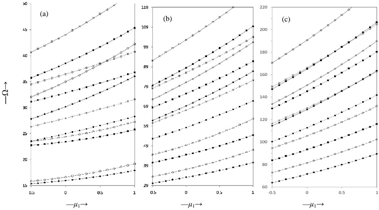
Fig. 3: Frequency parameter for C-C, C-S and C-F plates vibrating in (a) first mode (b) second mode and (c) third mode, for  $a/b = 1$ ,  $\mu_2 = 0.5$ ,  $K=0.02$ ,  $\alpha_1=0.5$ . ———, C-C; - - - - - , C-S; - - - - - , C-F; ■,  $\beta = -0.5$ ,  $\alpha_2 = -0.3$ ; □,  $\beta = -0.5$ ,  $\alpha_2 = 0.3$ ; ●,  $\beta = 0.5$ ,  $\alpha_2 = -0.3$ ; ○,  $\beta = 0.5$ ,  $\alpha_2 = 0.3$ .
