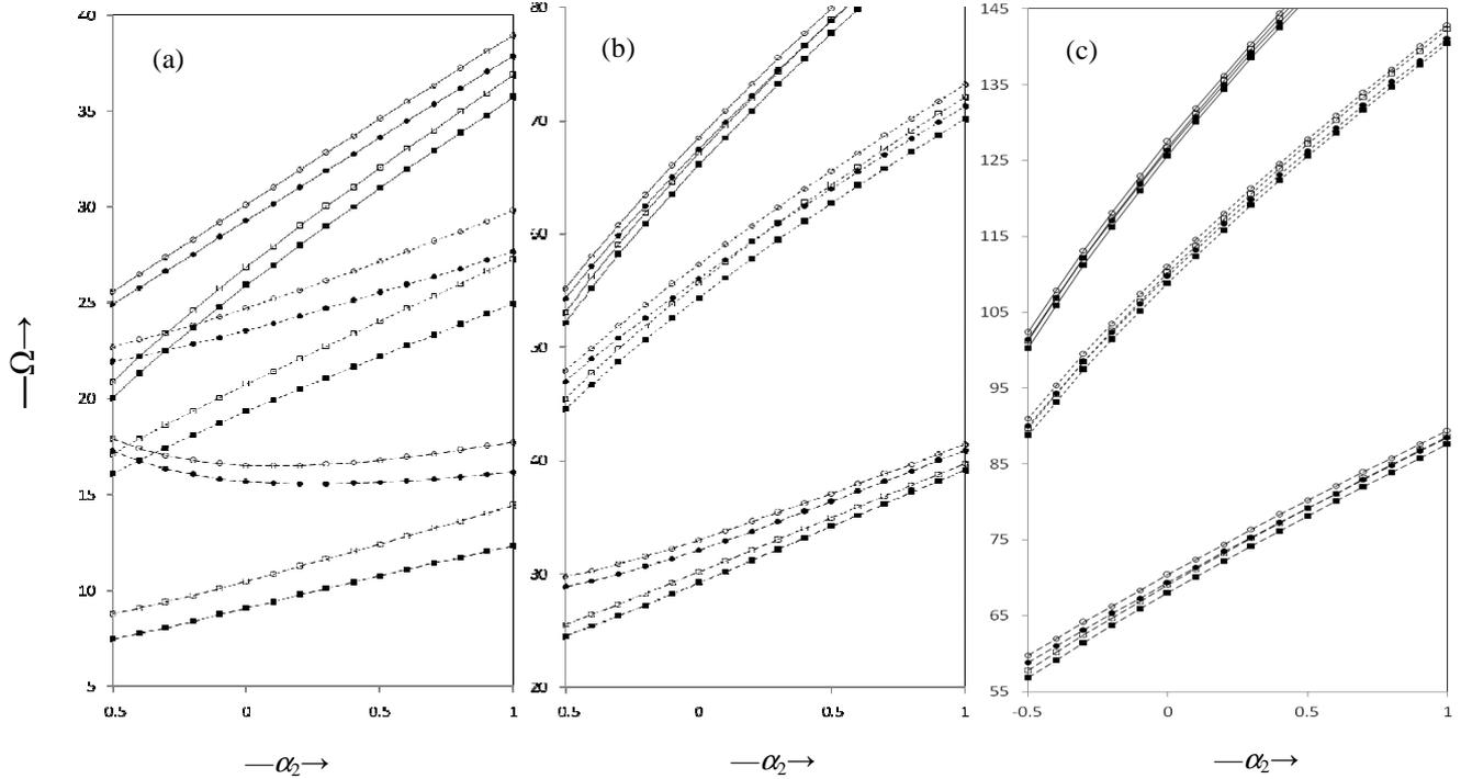
Fig. 8: Frequency parameter for C-C, C-S and C-F plates vibrating in (a) first mode (b) second mode and (c) third mode, for  $a/b=1, \beta=0.5, \mu_2=0.5, \alpha_1=0.0$ . ———, C-C; -----, C-S; - - - - -, C-F;  $\blacksquare$ ,  $\mu_1 = -0.5, K=0.00$ ;  $\square$ ,  $\mu_1 = 0.5, K=0.0$ ;  $\bullet$ ,  $\mu_1 = -0.5, K=0.02$ ;  $\circ$ ,  $\mu_1 = 0.5, K=0.02$ .
