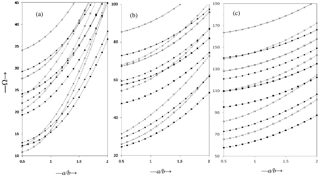
Fig. 6: Frequency parameter for C-C, C-S and C-F plates vibrating in (a) first mode (b) second mode and (c) third mode, for  $\beta = 0.5$ ,  $\mu_2 = 0.5$ ,  $K=0.02$ ,  $\alpha_1=0.5$ . ———, C-C; - - - - - , C-S; - - - - - , C-F; ■,  $\mu_1 = -0.5$ ,  $\alpha_2 = -0.3$ ; □,  $\mu_1 = -0.5$ ,  $\alpha_2 = 0.3$ ; ●,  $\mu_1 = 0.5$ ,  $\alpha_2 = -0.3$ ; ○,  $\mu_1 = 0.5$ ,  $\alpha_2 = 0.3$ .
