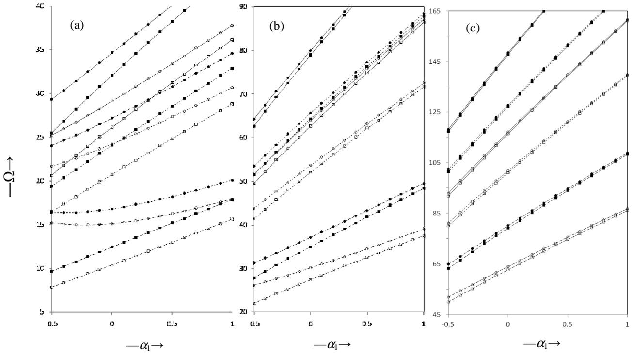
Fig. 7: Frequency parameter for C-C, C-S and C-F plates vibrating in (a) first mode (b) second mode and (c) third mode, for  $a/b=1, \beta=0.5, \mu_2=0.5, \alpha_2=0.0$ . ———, C-C; -----, C-S; - - - - -, C-F;  $\blacksquare$ ,  $\mu_1 = -0.5, K=0.00$ ;  $\square$ ,  $\mu_1 = 0.5, K=0.0$ ;  $\bullet$ ,  $\mu_1 = -0.5, K=0.02$ ;  $\circ$ ,  $\mu_1 = 0.5, K=0.02$ .
