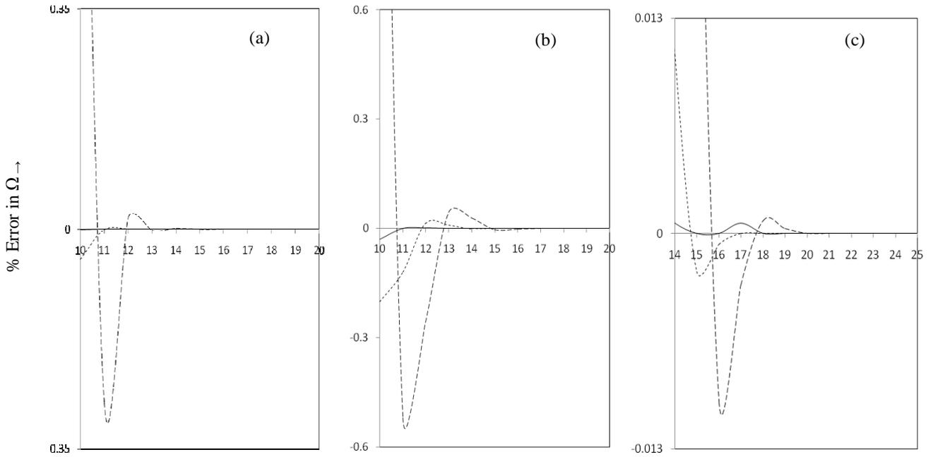
Fig. 2: Percentage error in frequency parameter  $\Omega$ ; (a) C-C plate (b) C-S plate and (c) C-F plate, for  $a/b=1.0$ ,  $K=0.02$ ,  $\mu_1=0.05$ ,  $\mu_2=-0.5$ ,  $\beta=0.5$ ,  $\alpha_1=-0.5$ ,  $\alpha_2=0.5$ , ———, first mode, -----, second mode, - - - -, third mode. % error =  $[(\Omega_m - \Omega_{20}) / \Omega_{20}] \times 100$ .
