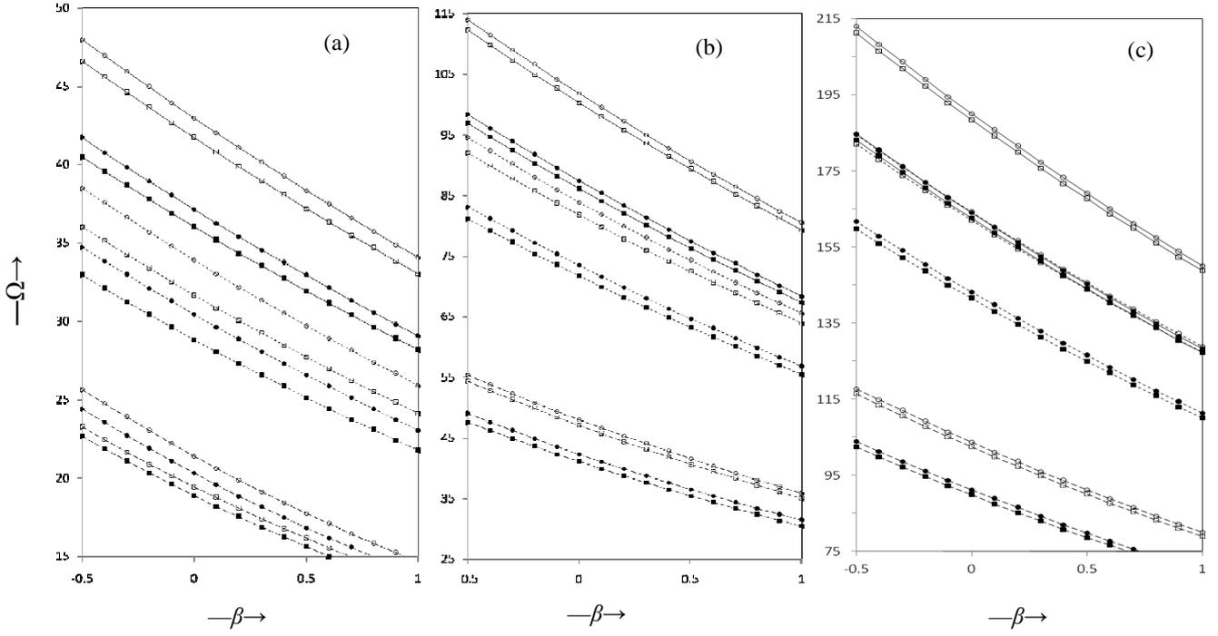
Fig. 5: Frequency parameter for C-C, C-S and C-F plates vibrating in (a) first mode (b) second mode and (c) third mode, for  $a/b = 1$ ,  $\mu_1 = 0.5$ ,  $K=0.02$ ,  $\alpha_1=0.5$ . ———, C-C; - - - - - , C-S; - - - - - , C-F; ■,  $\mu_2 = -0.5$ ,  $\alpha_2 = -0.3$ ; □,  $\mu_2 = -0.5$ ,  $\alpha_2 = 0.3$ ; ●,  $\mu_2 = 0.5$ ,  $\alpha_2 = -0.3$ ; ○,  $\mu_2 = 0.5$ ,  $\alpha_2 = 0.3$ .
