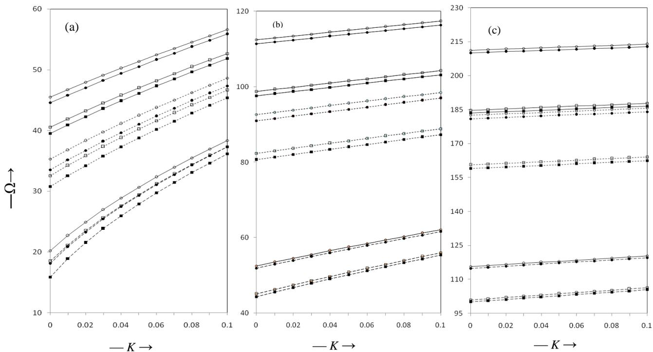
Fig. 9: Frequency parameter for C-C, C-S and C-F plates vibrating in (a) first mode (b) second mode and (c) third mode, for  $a/b=1, \beta=-0.5, \alpha_1=0.5, \alpha_2=0.5$ . ———, C-C; - - - - - , C-S; - - - - - , C-F; ■,  $\mu_1=-0.3, \mu_2=-0.3$ ; □,  $\mu_1=-0.3, \mu_2=0.3$ ; ●,  $\mu_1=0.3, \mu_2=-0.3$ ; ○,  $\mu_1=0.3, \mu_2=0.3$ .
