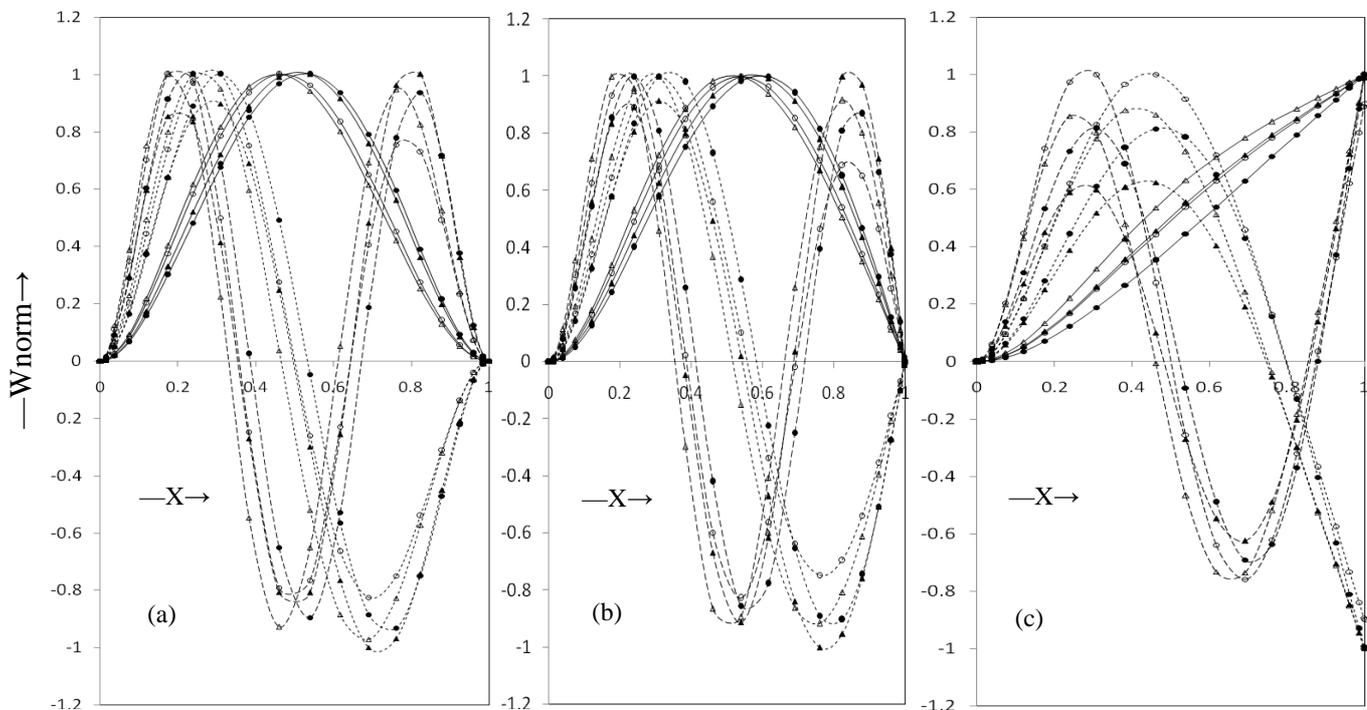
Fig. 10: Normalized displacements for the first three modes of vibration for (a) C-C plate (b) C-S plate and (c) C-F plate, for  $a/b=1.0, \alpha_1=0.5, K=0.02, \mu_1=-0.5, \mu_2=0.5$ . ———, first mode; - - - - - , second mode; - - - - - , third mode.  $\Delta, \beta=-0.5$ ; ○,  $\beta=0.5$ ;  $\blacktriangle, \bullet, \alpha_2=-0.3$ ;  $\triangle, \circ, \alpha_2=0.3$ .
