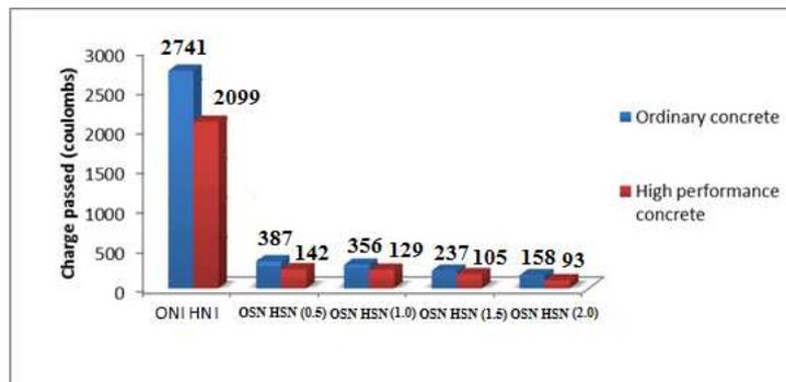
Figure 9. Rapid Chloride Permeability Test results
