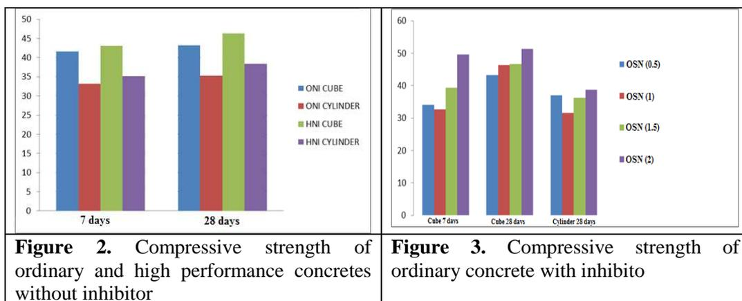
The compressive strength of cubes and cylinders of ordinary concrete with inhibitor at 7 days and at 28 days is shown in Fig.3. The compressive strength of cubes and cylinders of high performance concrete with inhibitor at 7 days and at 28 days and the test setup are shown in Fig.4.
