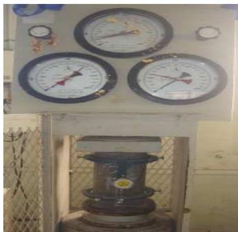
Figure 6a Test setup for Modulus of Elasticity of Concrete
