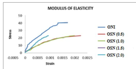
Figure 6b Stress Vs. Strain curve for ordinary concrete without and with inhibitor
