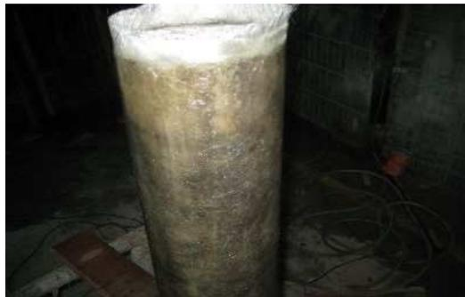
**Figure 3: Wrapped Specimens**
