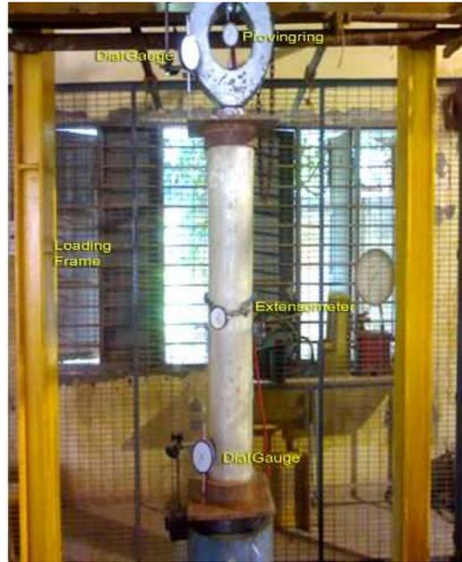
**Figure 4:** Test set-up with instruments
