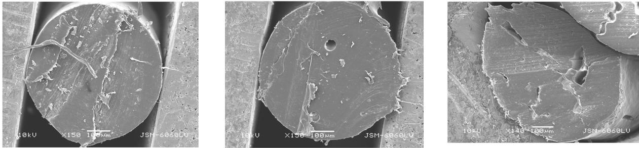
**Figure 8.** SEM micrographs of cross-section of monofilaments spun from: (a.) 100% virgin polymer, (b.) 85% virgin/15% recycled polymer blend and (c.) 50% virgin/50% recycled polymer blend
