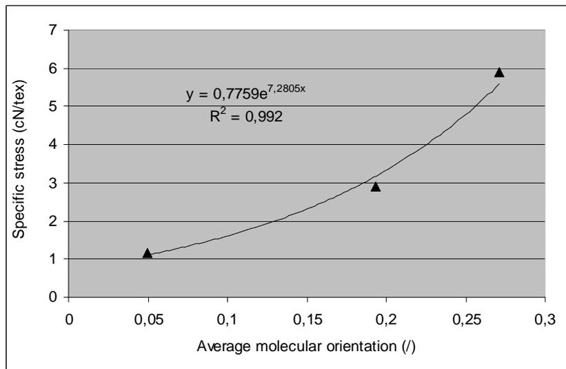
**Figure 10.** Specific stress of monofilaments versus average molecular orientation.
