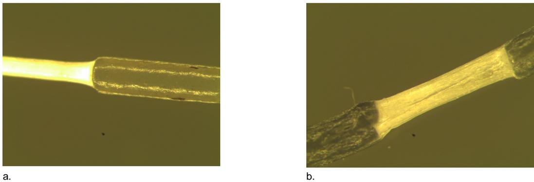
**Figure 5.** Longitudinal view obtained after drawing monofilaments spun from: (a.) 85% virgin/15% recycled polymer blend and (b.) 50% virgin/50% recycled polymer blend
