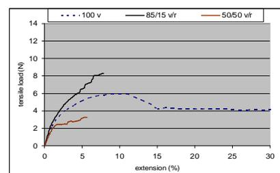
**Figure 6.** Load vs. extension curve of monofilaments spun from 100% virgin polymer (100 v), 85% virgin/15% recycled polymer blend (85/15 v/r) and 50% virgin/50% recycled polymer blend (50/50 v/r).
