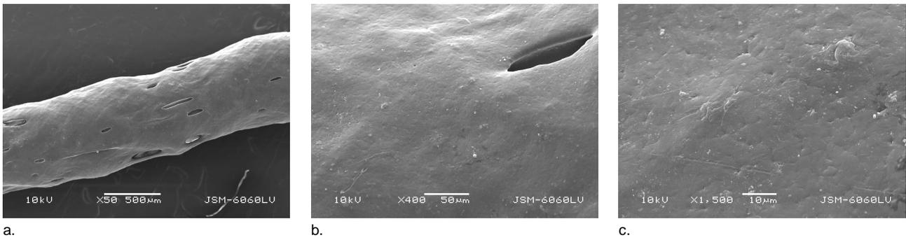
**Figure 3.** SEM micrographs of monofilaments spun from the 50% virgin/50% recycled polymer blend: (a.) 50x magnification, (b.) 400x magnification and (c.) 1500x magnification
