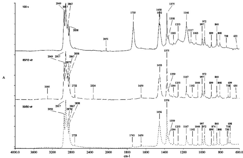
**Figure 9.** FTIR spectra of monofilaments spun from: (a.) 100% virgin polymer, (b.) 85% virgin/15% recycled polymer blend and (c.) 50% virgin/50% recycled polymer blend.
