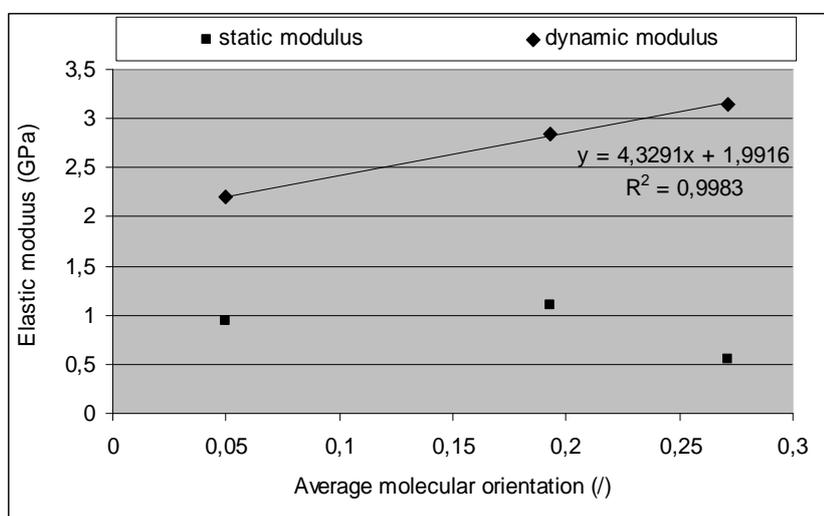
Figure 12. Elastic modulus of monofilaments versus average molecular orientation.
