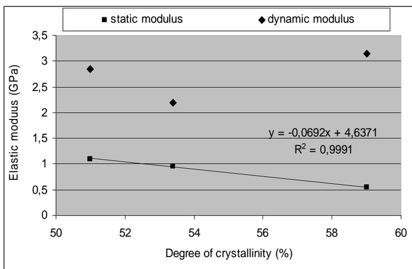
Figure 11. Elastic modulus of monofilaments versus degree of crystallinity.
