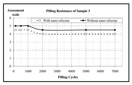
Figure 2. Pilling resistance of sample 3
