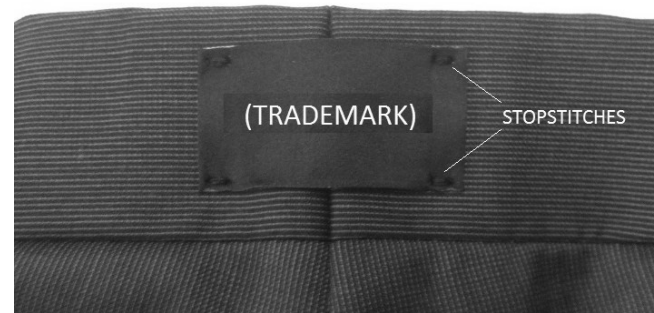
Figure 1. The Display of a Sewed Trademark Label to the Rear Center of a Trouser.
