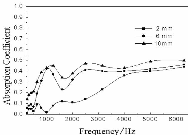
Fig. 3. Effect of thickness on sound absorption properties
