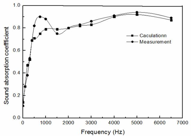
Fig. 8. Measurement and calculation of normal incidence sound absorption coefficients ( $\alpha$ ).
