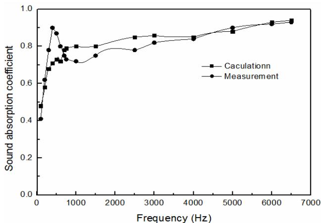
Fig. 7. Measurement and calculation of normal incidence sound absorption coefficients (I).
