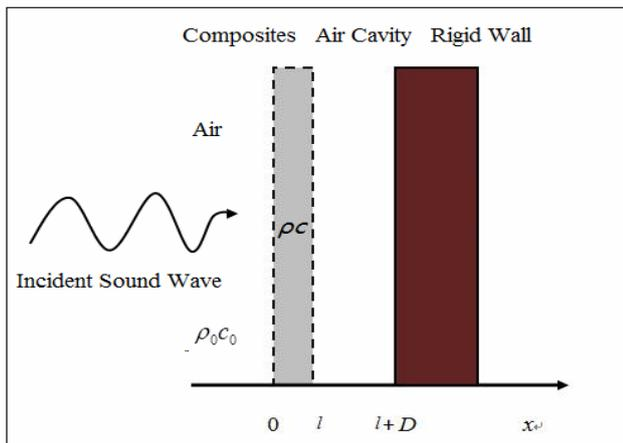
Fig.6. Illustration of the composites installation method (II).
