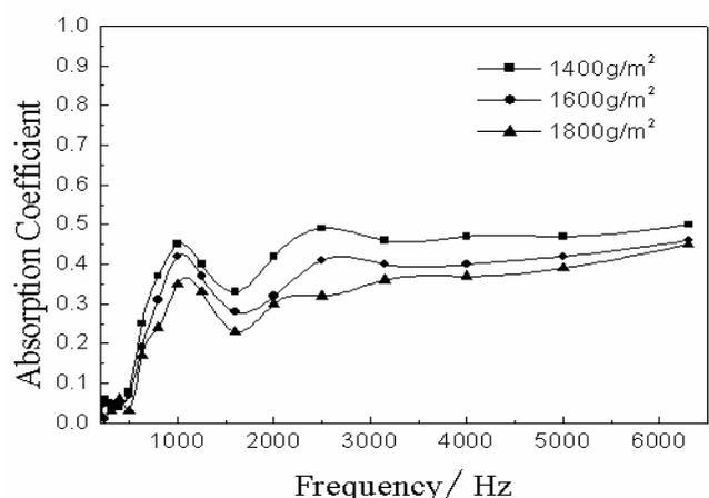
Fig.2. Effect of density on sound absorption properties
