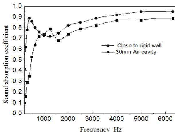
Fig.4. Effect of air cavity depth on sound absorption properties
