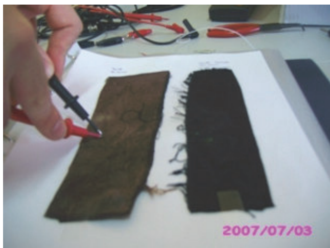
Figure 2. Measurement of electrical conductivity with two terminal technique
