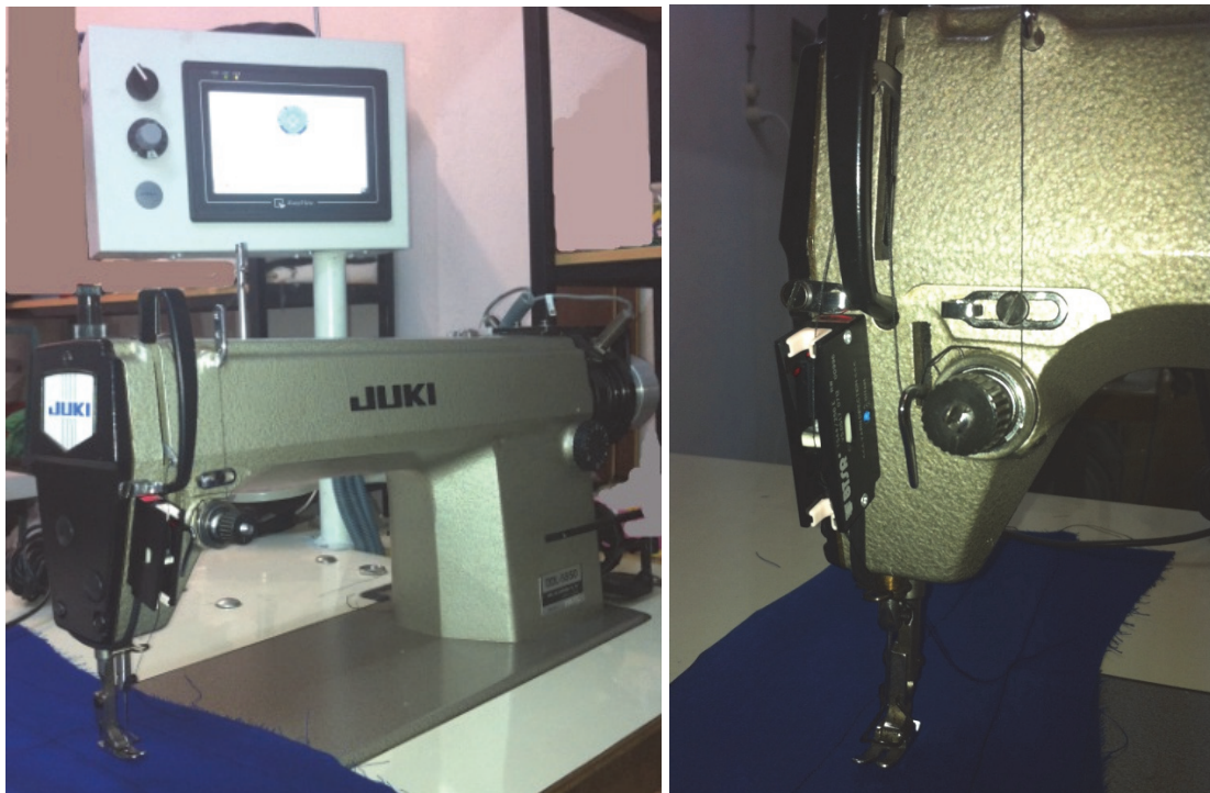
Figure 1. Sewing needle thread tension test system set-up on a Juki DDL-5550 model lockstitch sewing machine in the Uludag University Textile Engineering laboratory.
