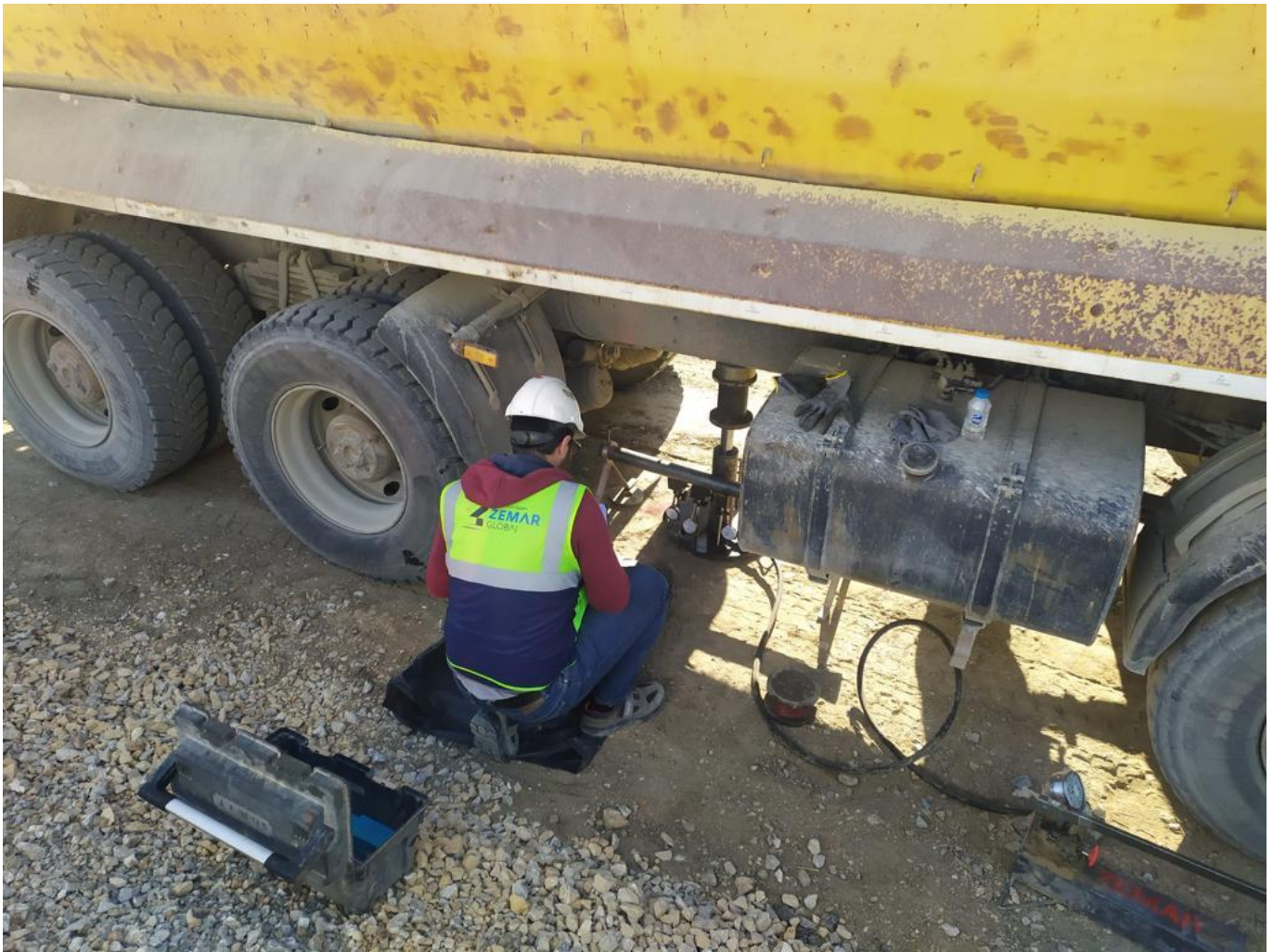
Figure 6. During Plate Load Testing- Field Photo
