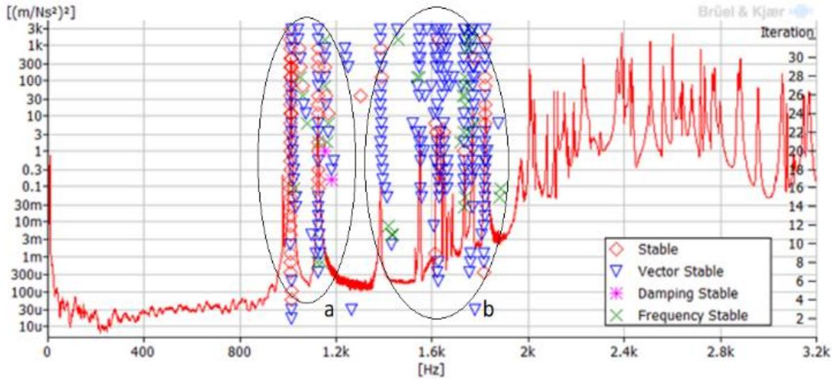
Figure 7. Stability Diagram of the Bladed Rotor
