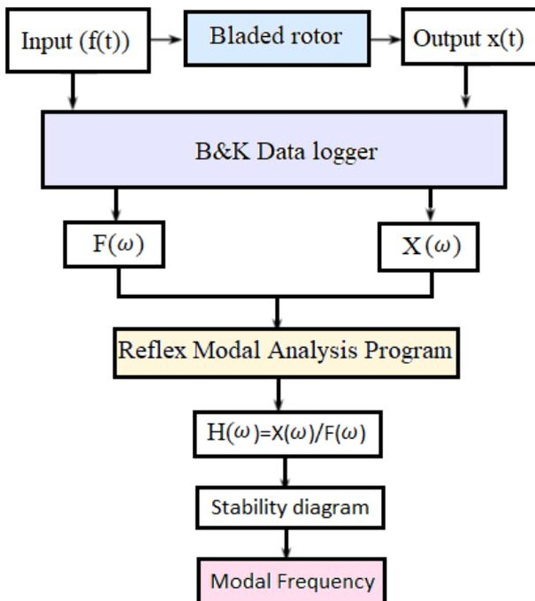
Figure 3. Schematic diagram of Experimental Modal Analysis
