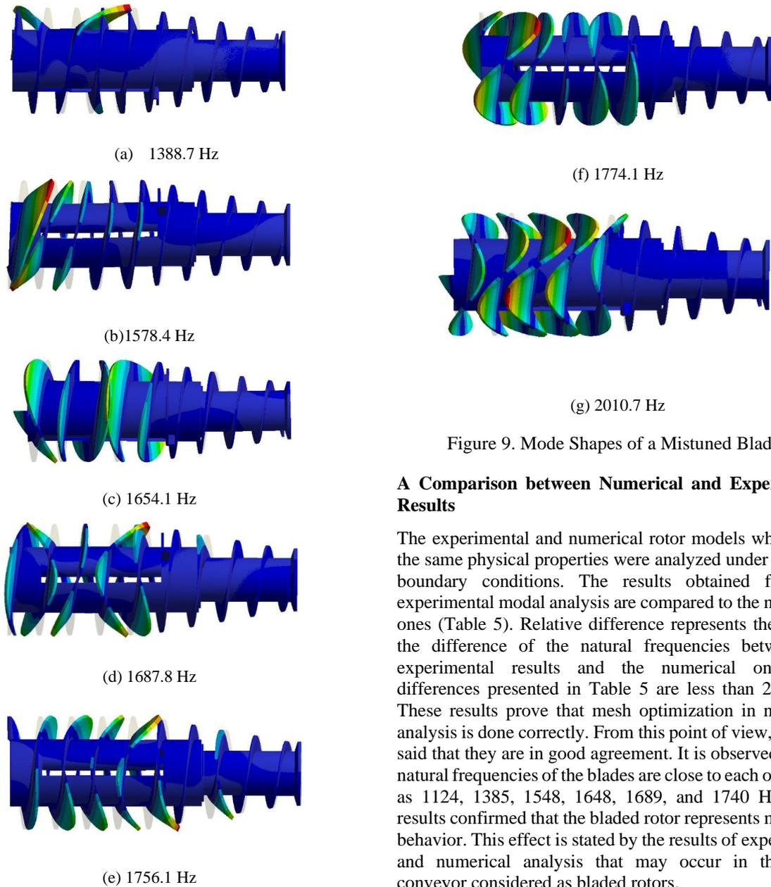
Figure 9. Mode Shapes of a Mistuned Blades
