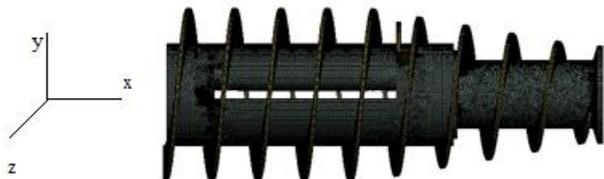
Figure 5. The Asymmetric Bladed Rotor Meshed Model
