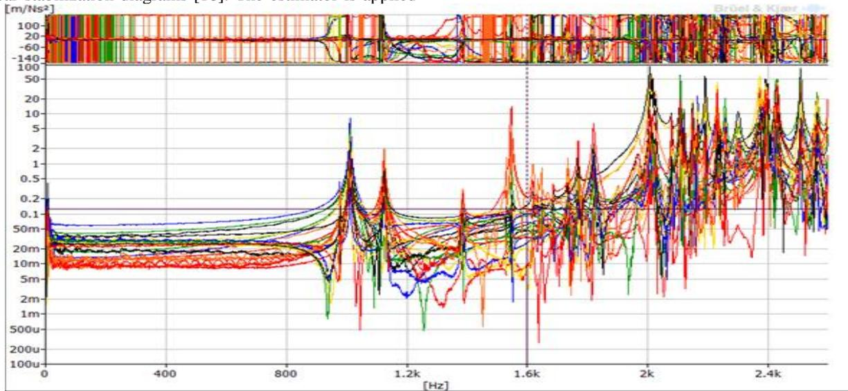
Figure 6. Frequency Response Functions for the Bladed Rotor
