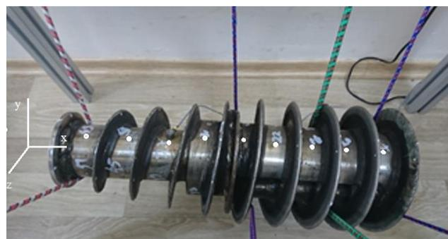
Figure 2. The Asymmetric Bladed Rotor with Free-Free Boundary Conditions
