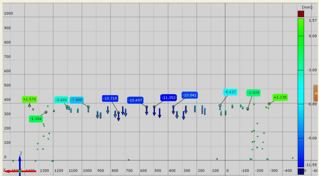
Figure 10. Displacement distribution under the 600 N load measured with GOM Tritop
