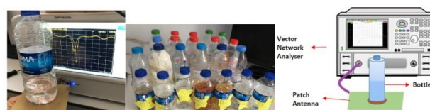
Figure 2. Experimental setup for liquid classification.
