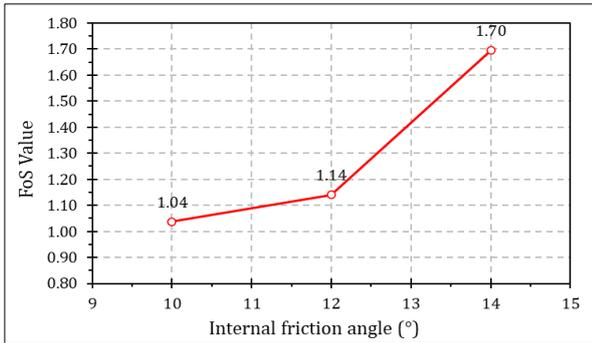
**Figure 12.** FoS number depending on internal friction angle
