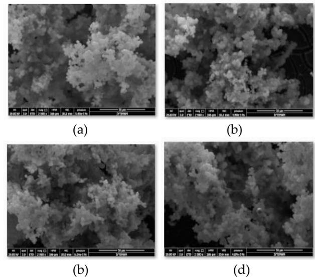
**Figure 2.** SEM images (2500X) of coatings obtained during waiting periods of a) 24 hours b) 48 hours c) 72 hours d) 96 hours in SBF
