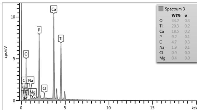
**Figure 5.**EDS analysis results for coating surfaces obtained
