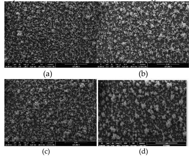
**Figure 1.** SEM images (100X) of coatings obtained during waiting periods of a) 24 hours b) 48 hours c) 72 hours d) 96 hours in SBF
