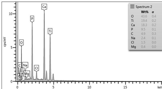
**Figure 4.**EDS analysis results of coating surfaces obtained by waiting for 48 hours in SBF
