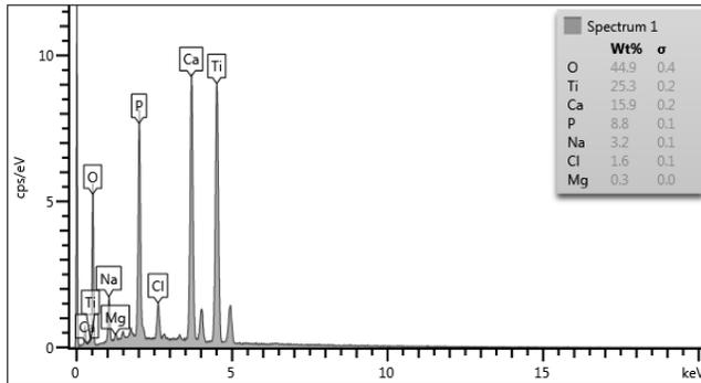
**Figure 3.**EDS analysis results of coating surfaces obtained by waiting for 24 hours in SBF
