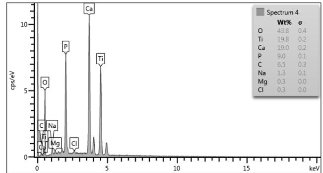
**Figure 6.**EDS analysis results for coating surfaces obtained by waiting for 96 hours in SBF
