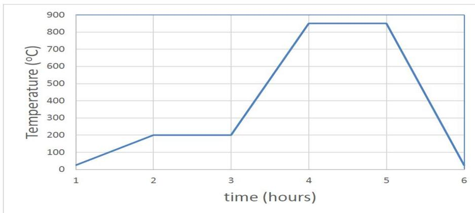
**Figure 4.** Sintering Temperature-Time
