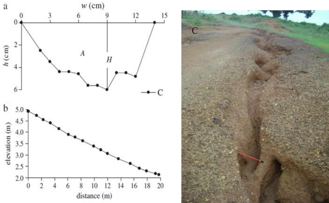
Figure 2. Example of the relief of (a) a rill cross section and (b) rill profile, (c) View of the Rill-C surveyed at Rangamati, Medinipur (after Stefano et al., 2013)
