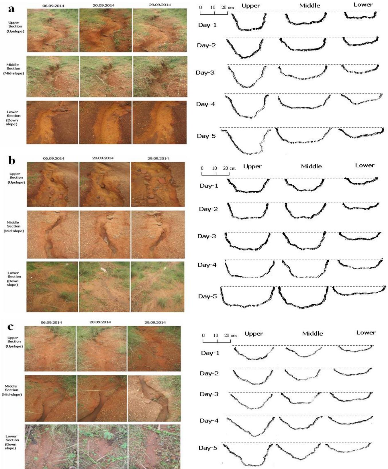
Figure 6. Rill erosion during 06.09.2014 and 29.09.2014 with field photo corresponding cross-sections, (a) Rill-A (b) Rill-B, and (c) Rill-C
