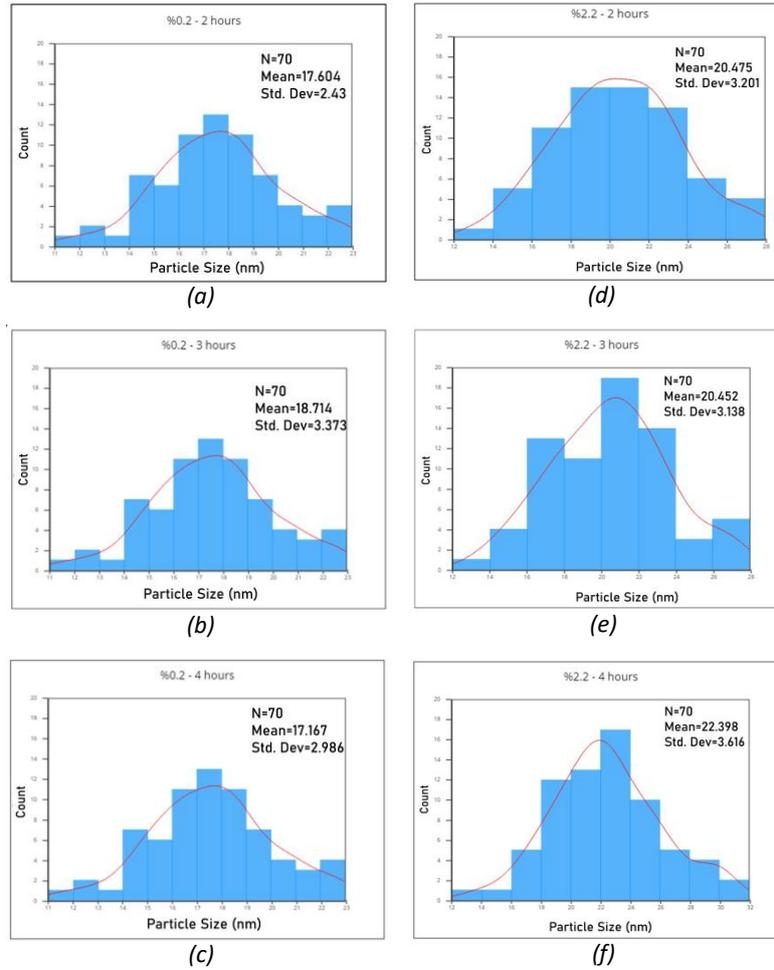
**Figure 4.** Size distribution curves of 0.2% w/w genipin crosslinked HSA nanoparticles for **a)** 2 h, **b)** 3 h and **c)** 4h; 2.2% w/w genipin crosslinked HSA nanoparticles **d)** 2 h; **e)** 3 h and **f)** 4 h.
