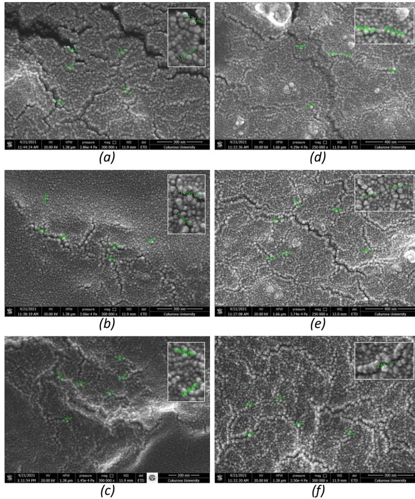
**Figure 3.** SEM images of 0.2% w/w genipin crosslinked HSA nanoparticles for **a)** 2 h, **b)** 3 h and **c)** 4 h; 2.2% w/w genipin crosslinked HSA nanoparticles **d)** 2 h; **e)** 3 h and **f)** 4 h
