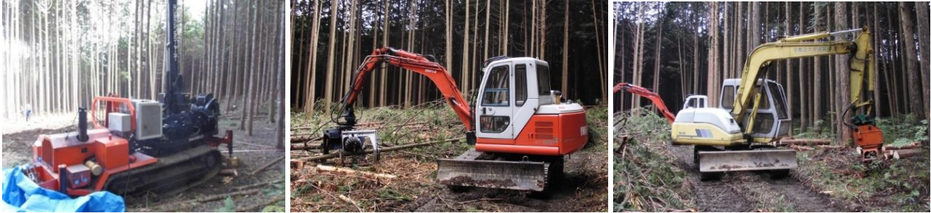
Figure 4. Forestry machines (Left: tower yarder, middle: processor, right: grapple loader)
