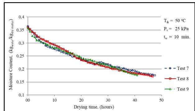
**Fig. 4.** Variation of moisture content with drying time for different operating pressure
