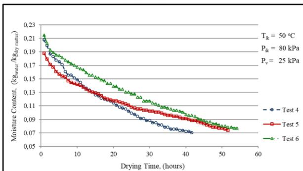
**Fig. 3.** Variation of moisture content with drying time for residence time in vacuum
