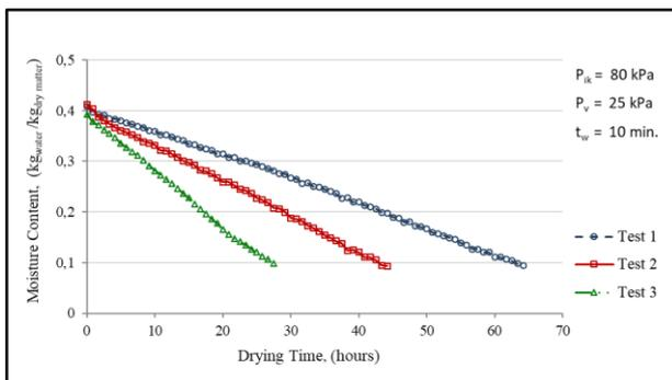
**Fig. 2.** Variation of moisture content with drying time for different drying temperature
