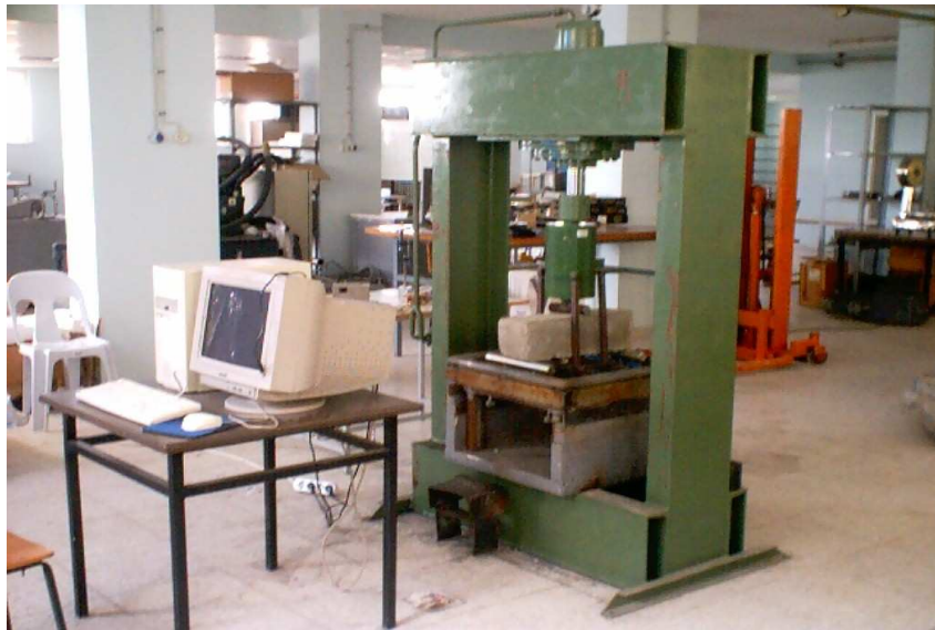
Picture 1. The loading frame with a capacity of 300 kN.
