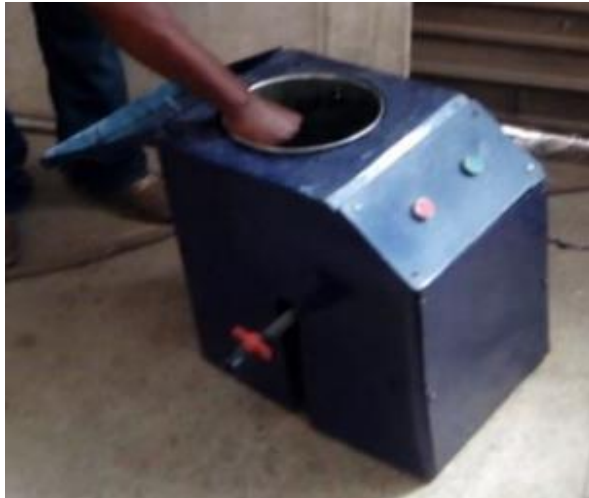
Fig. 6 Fabricated prototype modular bitter leaf washing and extraction machine
