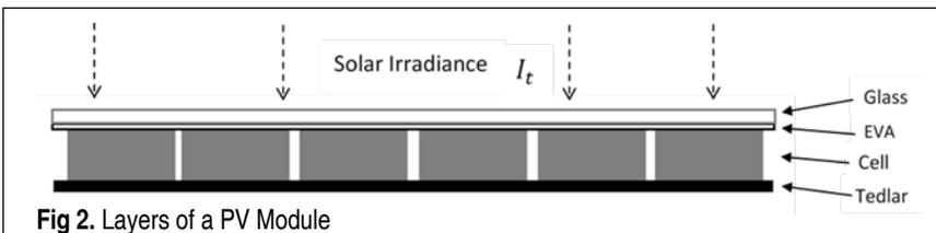
**Fig 2.** Layers of a PV Module
