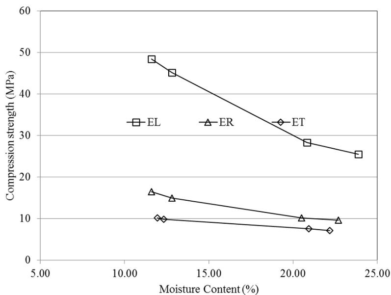
Figure 4. Influence of MC on Compression strength in three orthotropic directions of sessile oak
