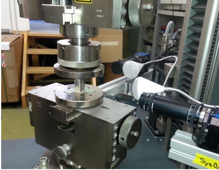
Figure 1. Compression test set up.
