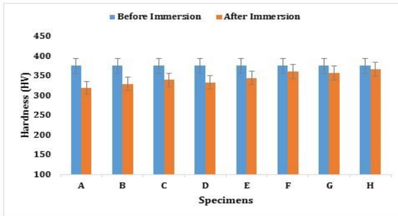
Fig. 11 Hardness of API L5 X60 specimens before and after corrosion
