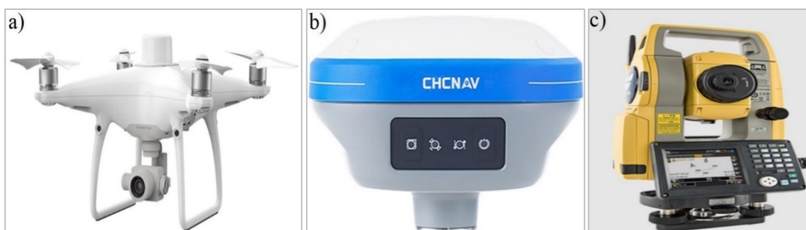
Figure 2. Measurement equipment used in the study: a) UAV; b) CORS; c) Total Station.
