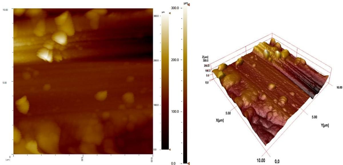
Fig.2 AFM images of (a) Pt/PPy-pTS electrode and (b) Pt/PPy-pTS-uricase electrode
