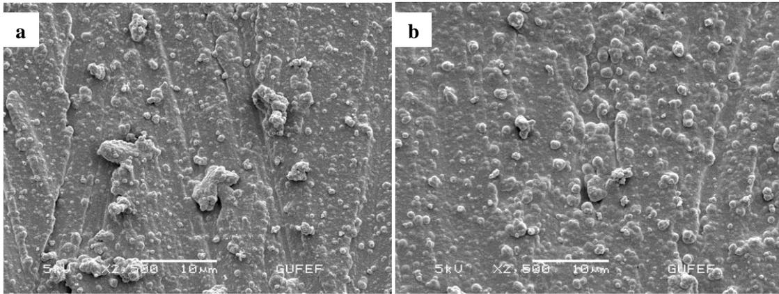
Fig.1 SEM images of (a) Pt/PPy-pTS electrode and (b) Pt/PPy-pTS-uricase electrode
