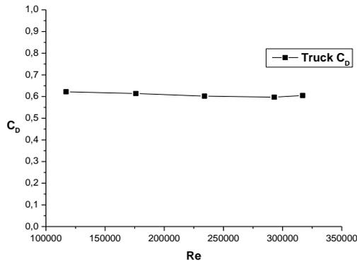
Fig. 8. The drag coefficient graphic of truck
