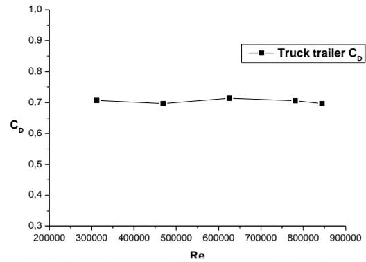
Fig. 9. The drag coefficient graphic of truck trailer
