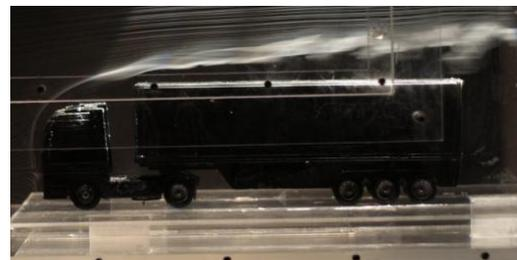
Fig.10. Flow visualization of truck and trailer
