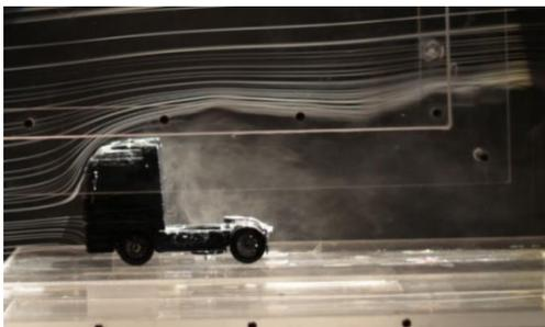
Fig.9. Flow visualization of truck
