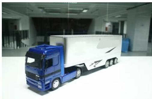
Fig. 3. 1/32 Scaled model vehicle
