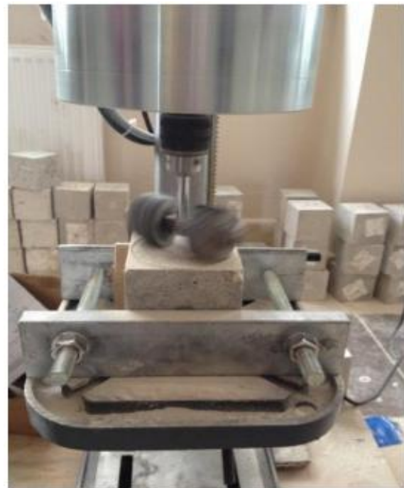
Figure 4. Abrasion resistance machine
