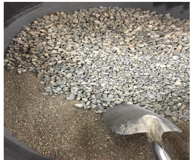
Figure 3. Sand and aggregate produced with demolished waste concrete
