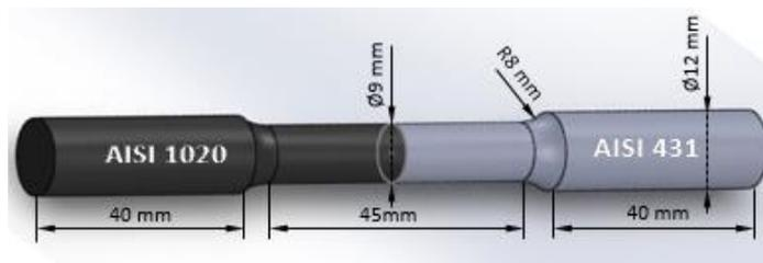
**Figure 4.** The sizes of tensile test sample.
