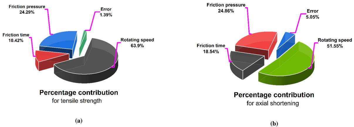
Figure 13. Percentage contributions; tensile strength (a) and axial shortening (b).
